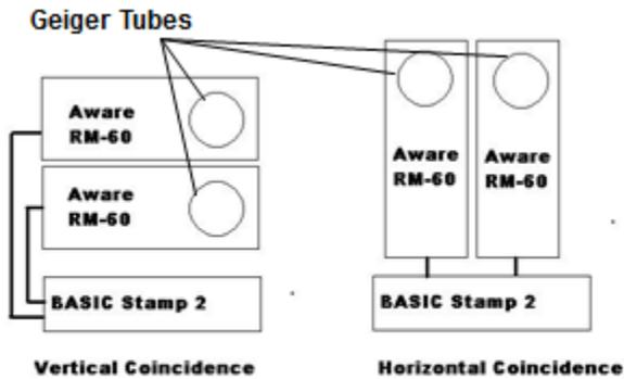
**Figure 1. Dual Geiger Counter Arrays** *Block diagrams of dual Geiger counter arrays*
