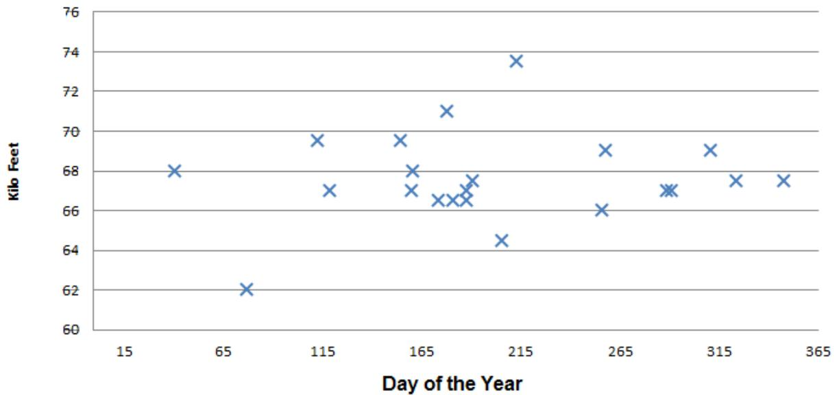
**Figure 6. Pfozter Maximum Altitude throughout the year** *The data shows the altitude of the Pfozter Maximum for several flights. Day 15 is January 15, There have been few flights during the winter because of the long flight paths that occur with the strong stratospheric jet stream during that time of the year.*
