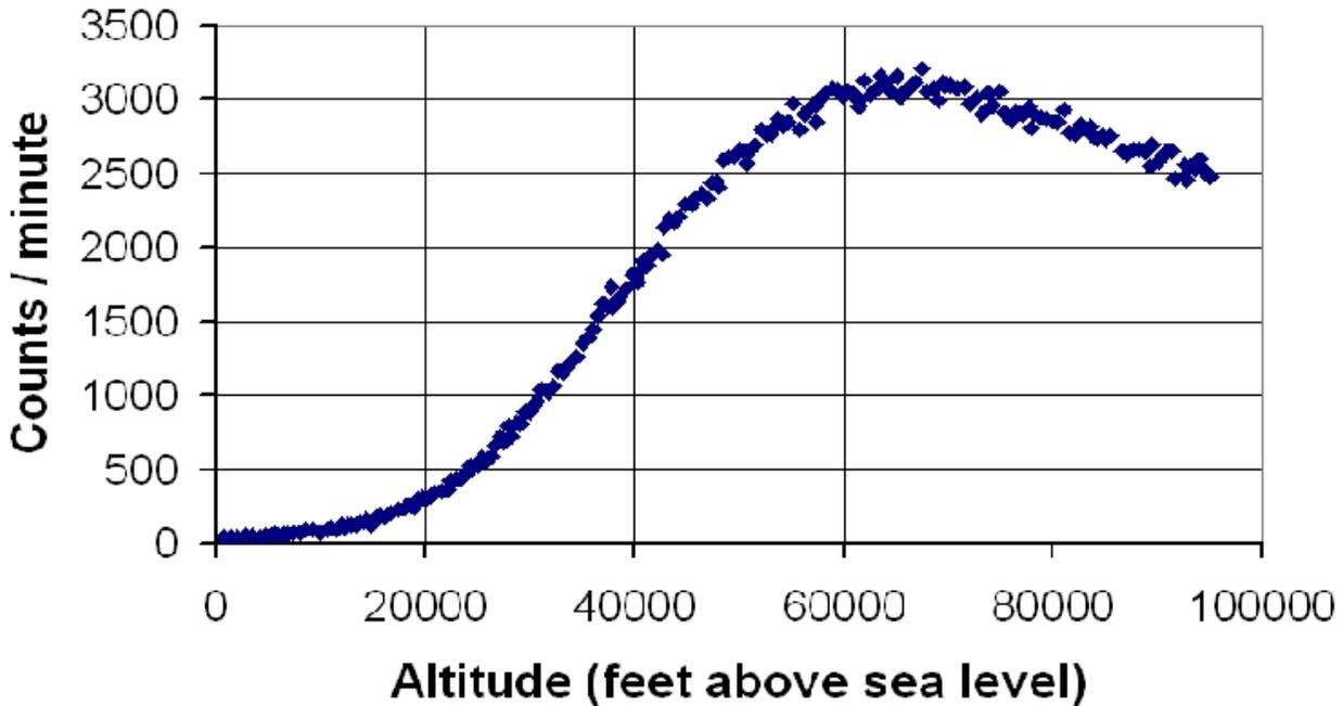
**Figure 5. Geiger counts versus altitude** Data from BASE 19 flight showing total Geiger counts versus altitude. The peak count rate occurs at an altitude between 60,000 and 70,000 feet. This peak is known as the Pfozter Maximum.
