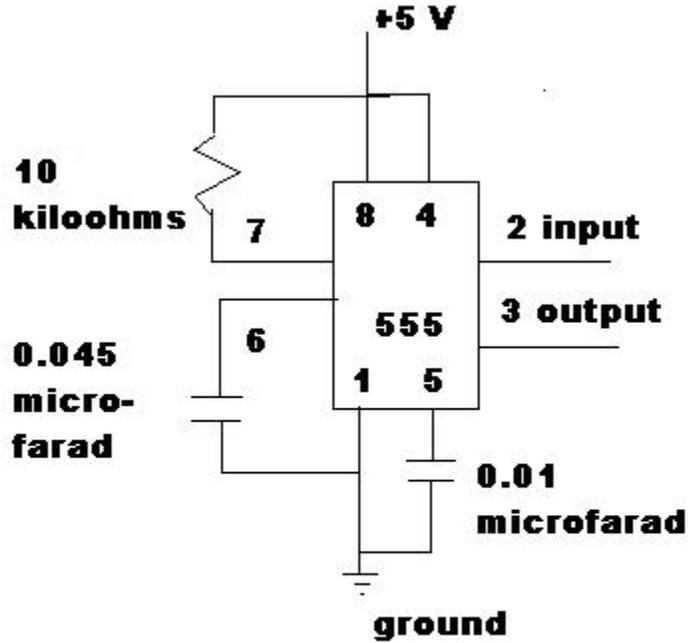
**Figure 4. 555 One-Shot Timing Circuit Schematic diagram of 555 timing circuit. Input from Geiger counter goes into pin 2 and output to counting program comes out on pin 3. The RC time constant is determined by the resistor on pin 7 and the capacitor on pin 6.**
