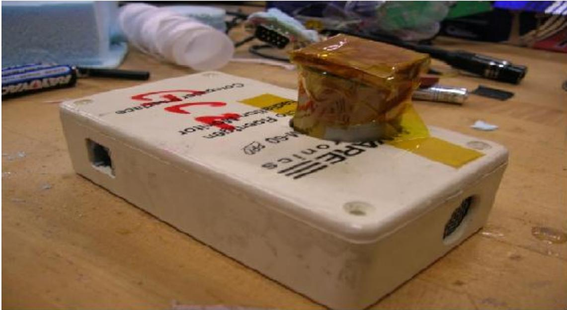
**Figure 9. Modified RM-60 Geiger counter with lead shield** *The tube is rotated 90 degrees and the lead wraps only around the tube.*
