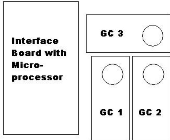
**Figure 2. Orthogonal Three Geiger Counter Array** *Block diagram of three Geiger counters in an orthogonal array. Horizontal coincidences measured by GC1 and GC2. Vertical coincidences measured with GC2 and GC2.*
