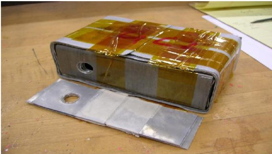
**Figure 8. Lead sheet enclosing the entire RM-60 Geiger counter.** *In 2010, DePauw students began a study of the effect of shielding the Geiger counter with lead.*
