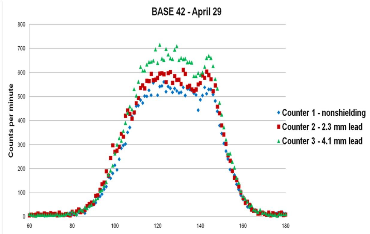
**Figure 10. Counts per minute versus time (in minutes) for lead shielded Geiger counters.** *Launch occurred at minute 60 with the burst just before minute 140. Note the much higher count rate for the thickest lead shield during the time that the Geiger counters were in the stratosphere.*
