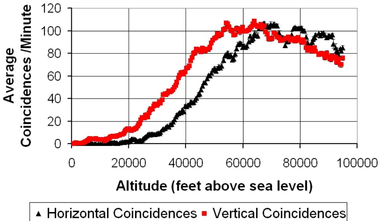
**Figure 7. Dual Geiger counter coincidences as a function of altitude from a typical flight.** *The coincidence data in average counts/minute shows a similar trend to the single Geiger counter data in Fig. 5. Note that the horizontal coincidences occur less frequently until the Geiger counters reach the portion of the stratosphere where the Pfozter maximum occurs.*
