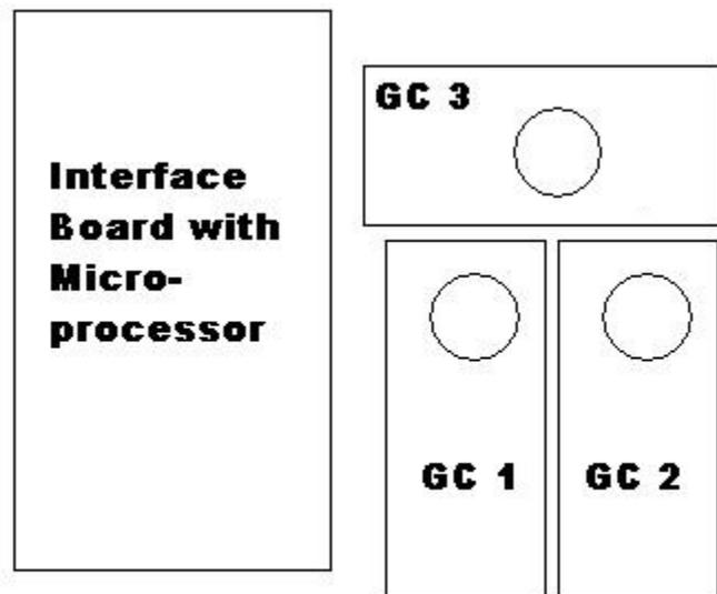
**Figure 3. Triple Geiger Counter Array for studying showers.** *Block diagram of three Geiger counters in non-orthogonal alignment.*
